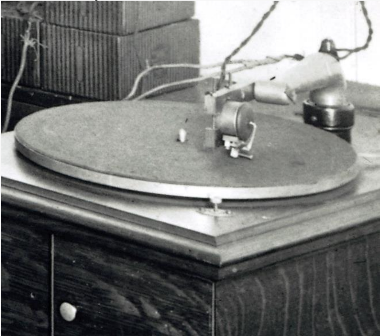
Fig. 5: Closeup of phonograph arm and “pickup” in the radio room in Fig. 1. Did Donald Little invent and fabricate the first transducer for turning record groove modulations into a varying voltage? Others had placed a mic in front of a phonograph’s horn or graphed a microphone element onto a portion of the phonograph’s acoustical linkage (tube) between the diaphragm and horn. (Getty Images)
